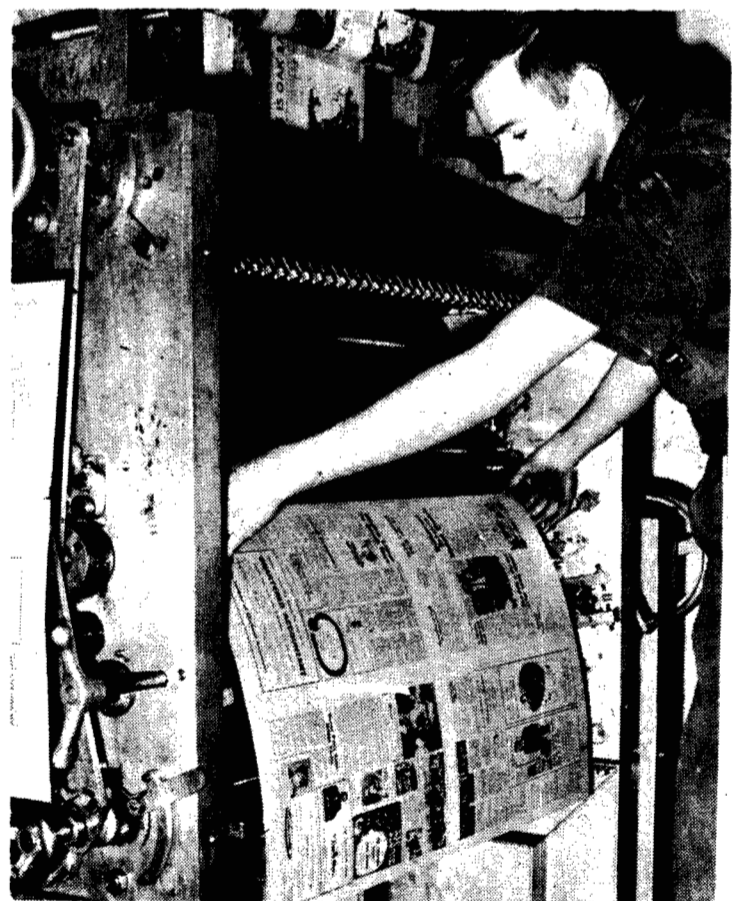
Step 9: The front page is fitted onto the offset press.
